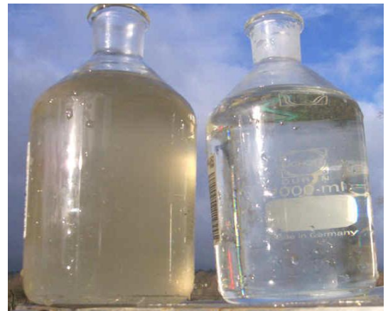
Figure 2 Typical Sewage effluent on the left and AFM filter media treated effluent on the right.
