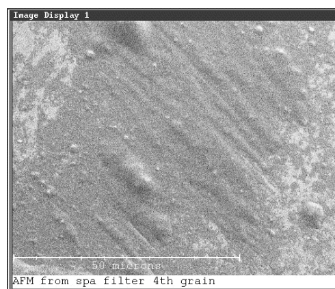
AFM after several years in a sewage treatment filter
